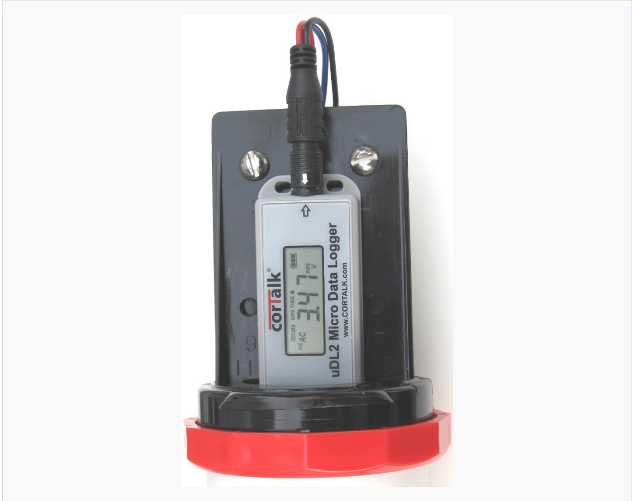
Figure 2 uDL2 Installed In a Test Station
