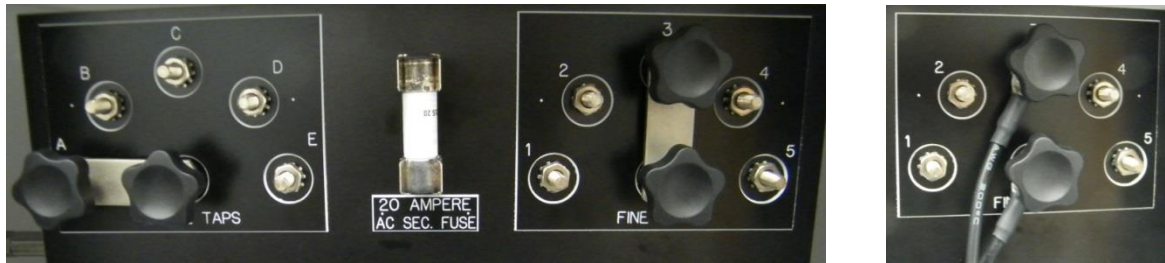
Figure 20 SRL1 Relay Contacts Installed In Series With Taps (Tap Bar Removed While In Use)
