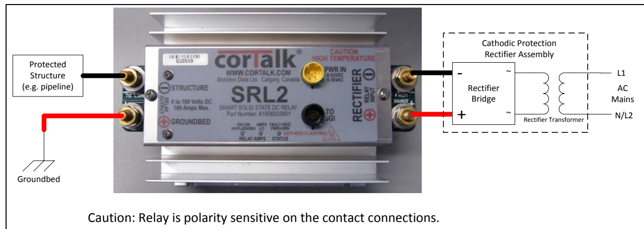
Figure 25 SRL2 Connections To Source and Load
