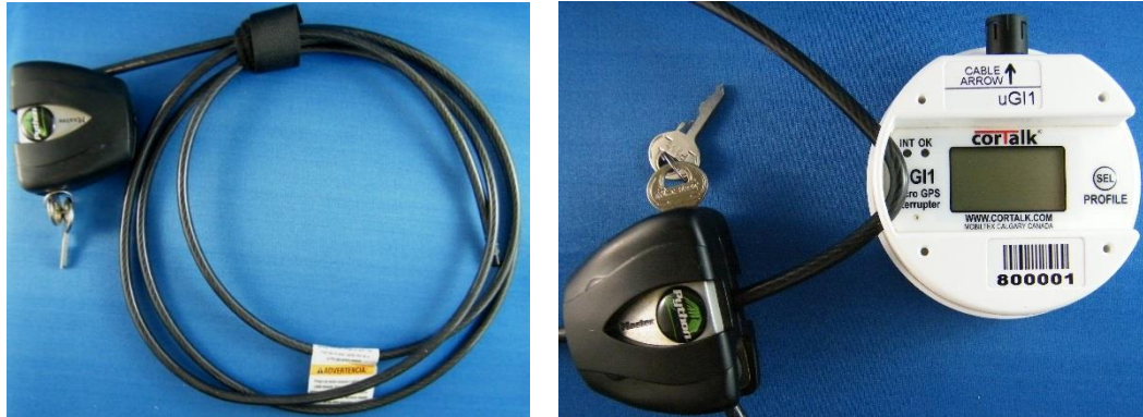
Figure 29 Master Lock 8417D Installation (Cable Fits Through uGI1 Lock Holes)
