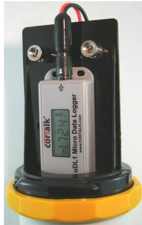
Positioned inside a CP test station
